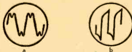
Fig. 3—Amplitude and harmonic distortion.
