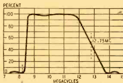
Fig. 1—Ideal shape of i.f. alignment curve.
